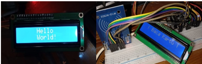
Fig. 10 16x2 led and rfid reader test results
